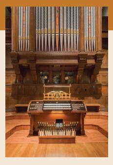
Six unison couplers with reversibles Solid State Organ Systems Multisystem with 100 memory levels, 10 generals, 6 divisionals, Organist Palette, and recording module Electric slider-pallet manual chests
